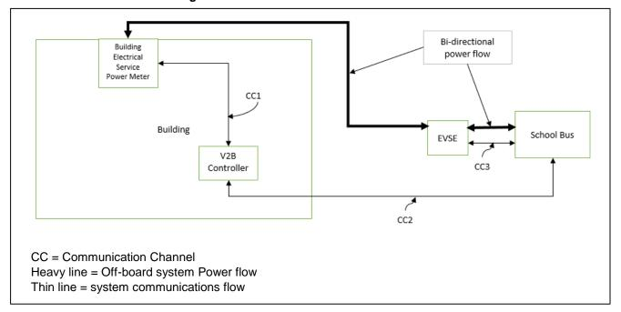
Figure 4: V2G Communication and Power Flow.
