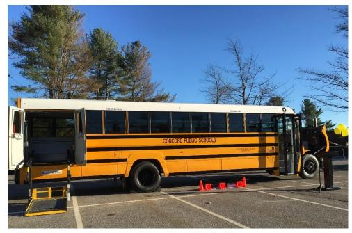
The wheel chair-accessible electric school bus deployed in Concord.
