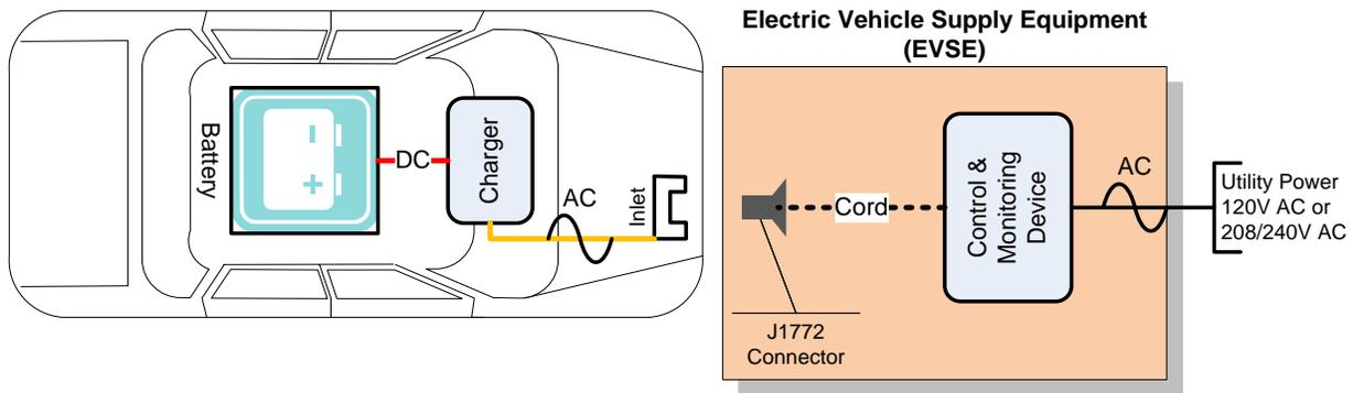
There are three distinct levels of EV charging in widespread use—Level 1 (120V), Level 2 (208 / 240 V), and DC fast charging (208-480 V). Table A-1 lists their specifications, and the subsequent sections provide further description. Using common standards for charging has greatly aided the adoption of EVs and the development of charging infrastructure. Figures A-2 through A-4 provide charging method examples.
